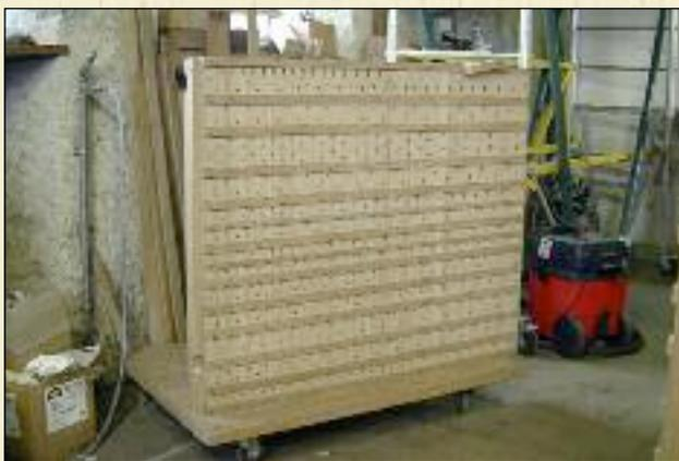
**Figure 1.5** Sound Board for the Recit-Positiv
