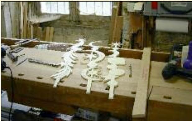
**Figure 1.10** Preliminary Models of the Carvings for the Top of the New Organ
