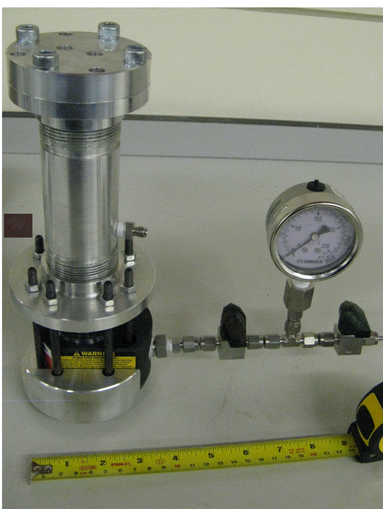
Figure 2: Triaxial test cell to house the sample along with pressure gauge and loading jack.
