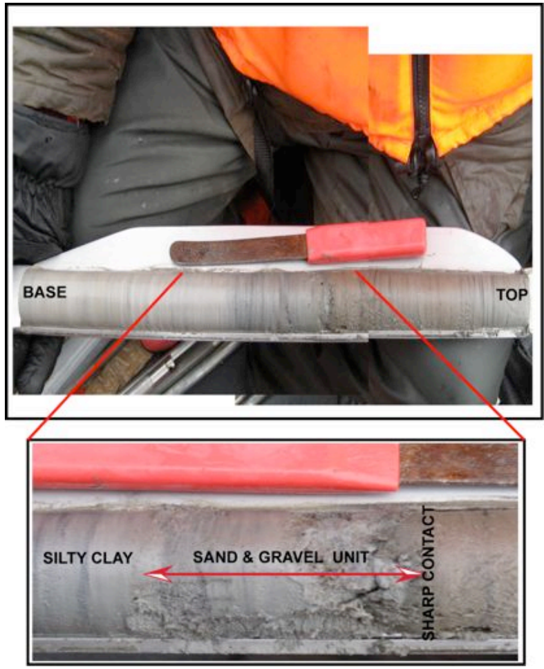
Seatter core 22 detailing the sand unit and associated upper organic unit and lower silty clays.
