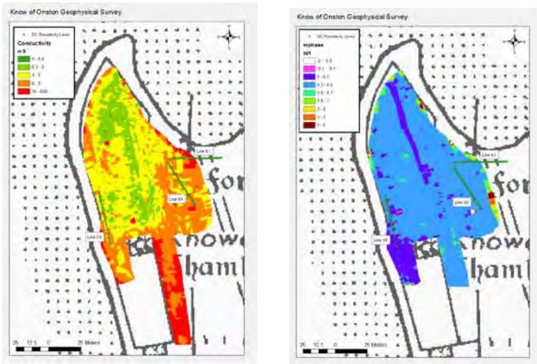
Figures 12 & 13: Ground Conductivity at Point of Onstan.
