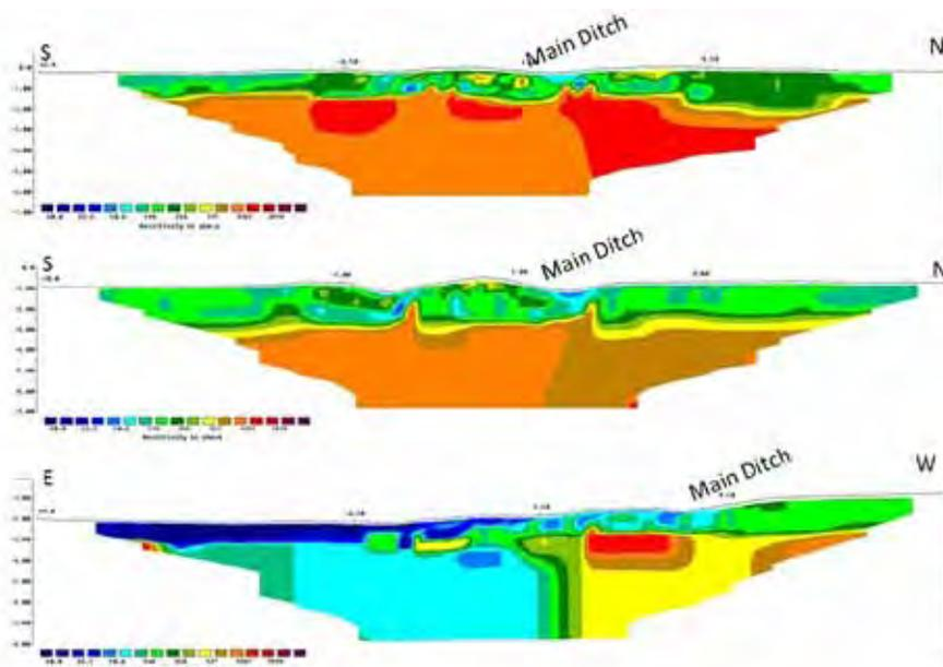
Figure 14: Resistivity variation across the ditch at Point of Onstan
