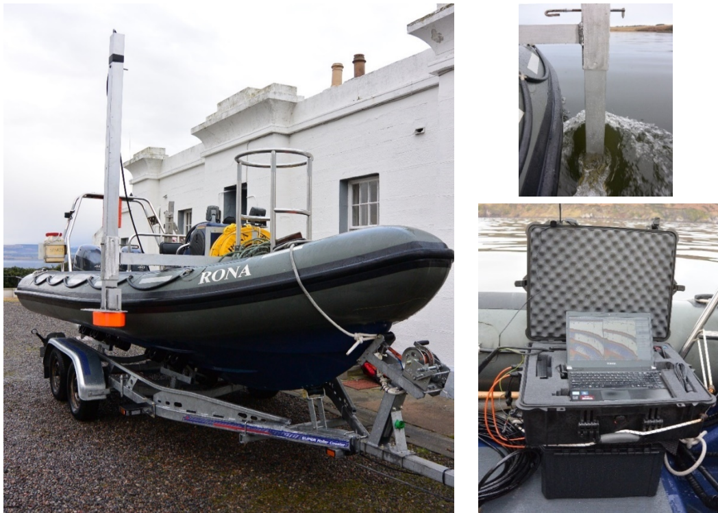
Figure 3.3: Pictures of the equipment used in the echo sounder surveys. Frame-mounted transducer on the RIB (left), transducer submerged during an acoustic transect (top right) and battery powered laptop and echo sounder during a survey (bottom right).
