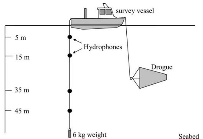
**Fig. 1** Design of the vertical 4-hydrophone array, showing the survey vessel, the dimensions of the array and the underwater drogue
