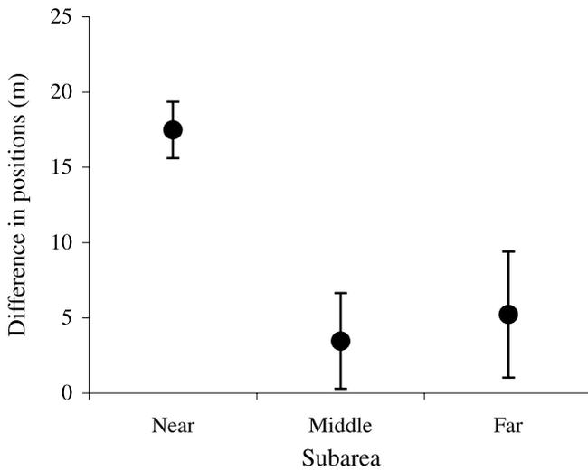
of the 20 subareas. The corresponding subareas were videotaped and the location of the boat was recorded regularly using an electronic theodolite. The locations of the boat were then estimated using the video technique and compared with those calculated using the theodolite. To assess the variation in accuracy with distance from the observation station, errors were compared between the far, middle, and near rows of subareas using a general linear model.
