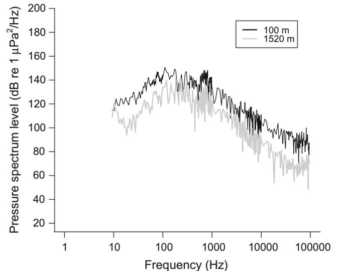
Fig. 4. Power spectral density of three seconds of pile-driving noise at 100 m and 1520 m distance. Recordings of pile-driving noise were made with Brüel and Kjaer 8104 and 8105 hydrophones. The data was over the frequency range 10 Hz to 96 kHz without correcting for sensitivity variations above 10 kHz.
