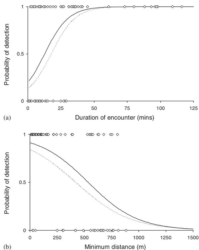
Figure 3. Changes in the probability of detection by a pair of T-PODs (solid line) and a single T-POD (dashed line) in relation to (a) the amount of time that the dolphin group spent in the area around the T-POD and (b) the group's minimum approach distance to the T-POD. Lines are fitted by logistic regression, all significant at  $P < 0.001$ . Raw data plotted as open diamonds.
