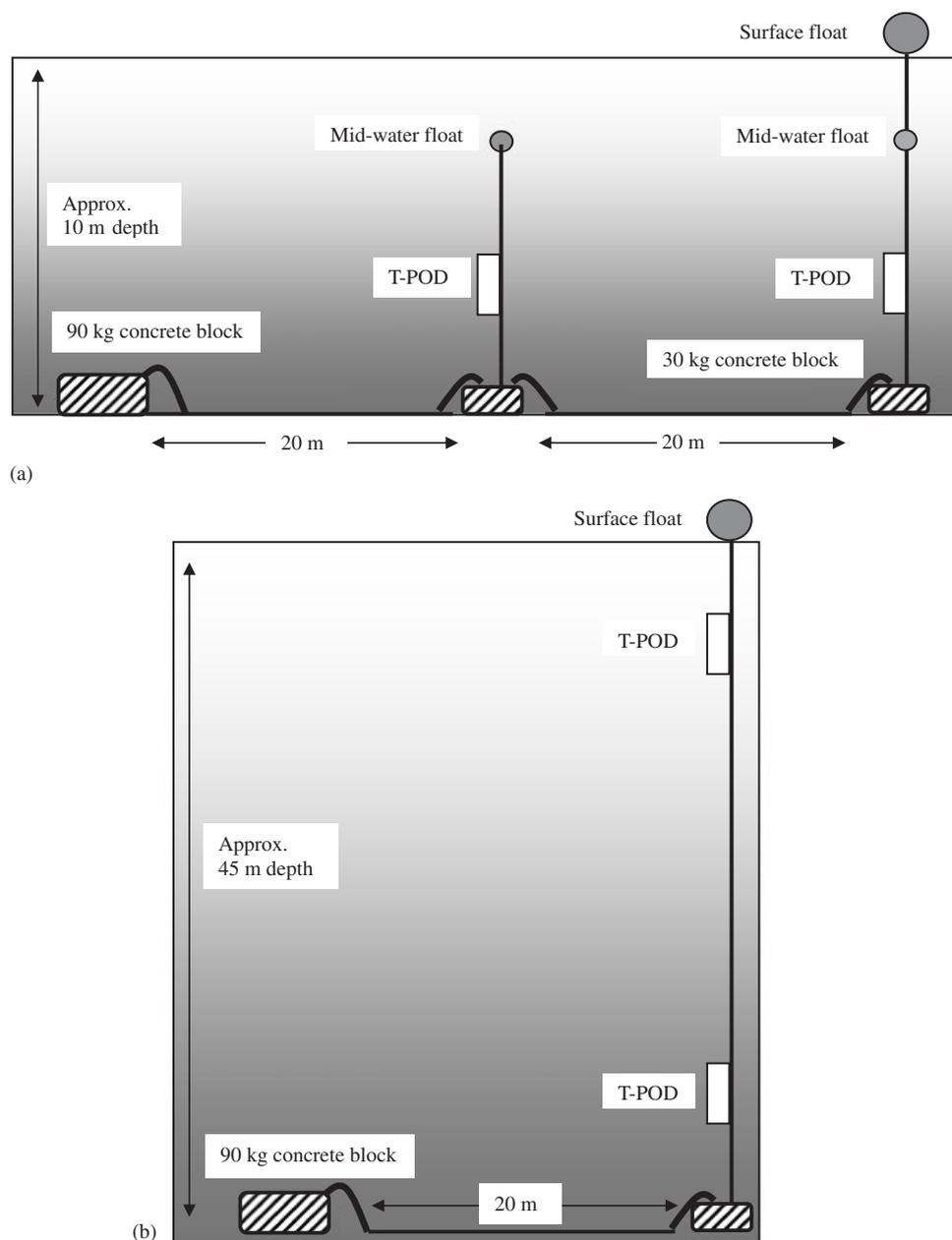
Figure 2. Schematic of (a) the T-POD shallow water moorings in the Cromarty Firth and Lossiemouth sites and (b) at the deeper water site in the outer Moray Firth.
