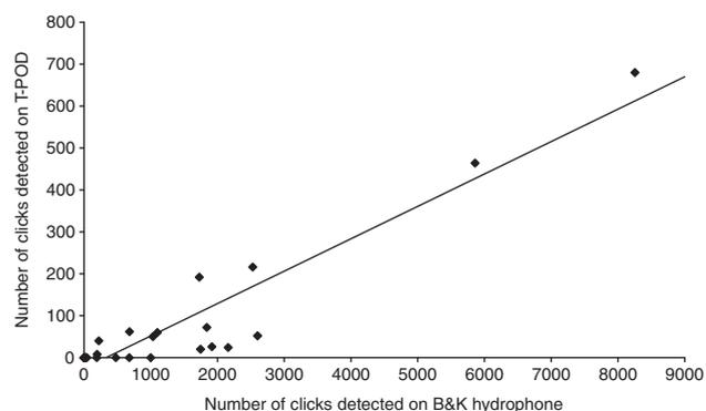
Figure 4. Relationship between the numbers of clicks recorded from the hydrophone and the numbers of clicks detected by the T-POD. Data are from 10-min sample recordings taken during boat surveys when dolphins were within 200 m of the survey vessel. Fitted line based on linear regression ( $F_{1,25} = 184.1$ ,  $P < 0.001$ ,  $r^2 = 0.88$ ).
