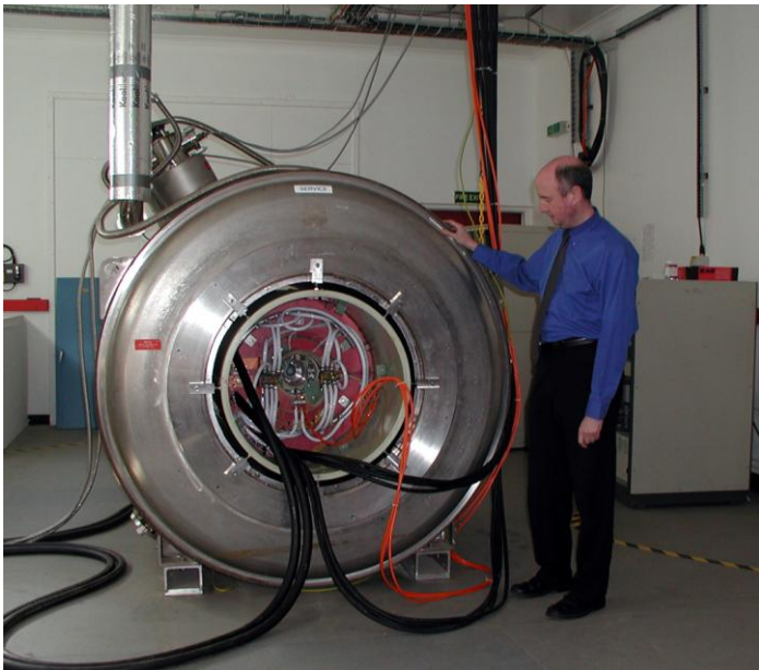
Figure 6: Left – schematic diagram showing end-view of 450 mT FFC-MRI magnet system. a:– 450 mT superconducting magnet generating field out of page; b:– active shield coil; c:– solenoidal configuration resistive field-offset coil, generating field up to 450 mT (anti-parallel or parallel to field of superconducting magnet); d:– gradient and shim coils. Right – photograph of 450 mT FFC-MRI magnet system, next to one of the authors (DJL).
