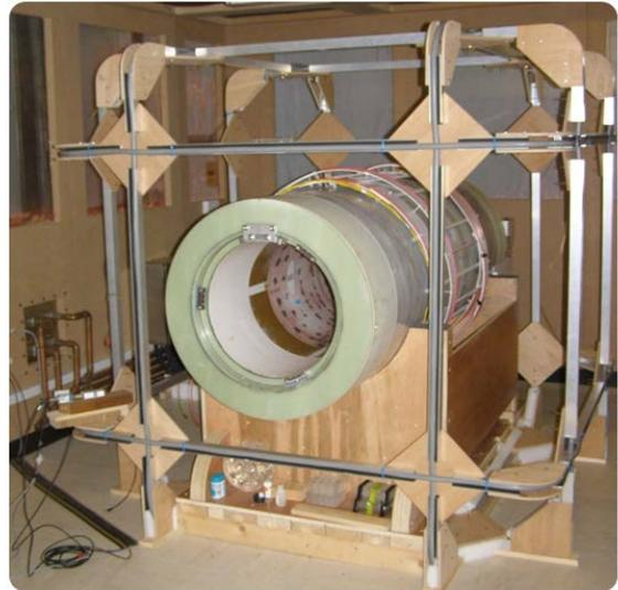
*Figure 2: 0.2 T FFC MRI scanner currently developed at Aberdeen. The main field is generated by the cylindrical magnet, which is surrounded by square coils designed for earth field compensation.*
