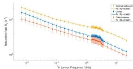
Fig. 3: Mean  $R_T$ -dispersion curves (Relaxation rate  $R_T=1/T_T$  versus  $^1\text{H}$  Larmor frequency  $\nu_0=\gamma/2\pi B_0^E$ ) of human glioblastoma and of pig WM (Corpus Callosum) and GM (Cortex). The errorbars correspond to one standard deviation. The fits were achieved using both the models presented in Eq. 1 and 2.
