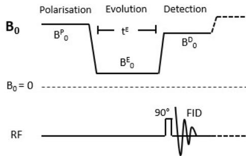
Fig. 1: FFC-NMR sequence for  $T_1$ -dispersion curves measurements.
