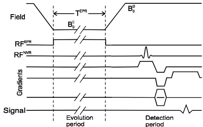
Figure 1: Field-Cycled PEDRI pulse sequence.
