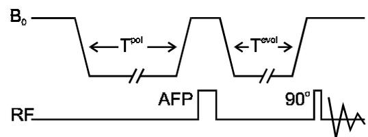
Figure 2: Field-Cycled IR pulse sequence.
