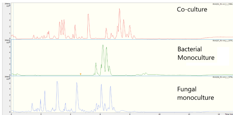
Figure 2: A comparison of the QTOF-HR-ESI-MS chromatograms of the fungal monoculture, bacterial monoculture, and their co-culture in short grain rice.
