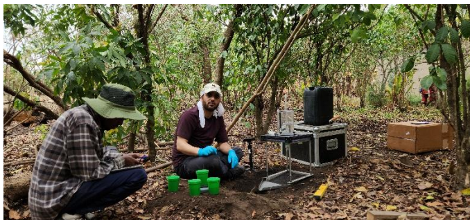
Measuring erosion using a portable rainfall simulator
