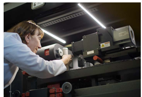
A robotic Particle Image Velocimetry System developed by the School is used in laboratory studies of flow dynamics, sediment transport and flow-biota interactions. The system's unique features include the flexibility to measure velocity fields at multiple locations and at various spatial scales.
