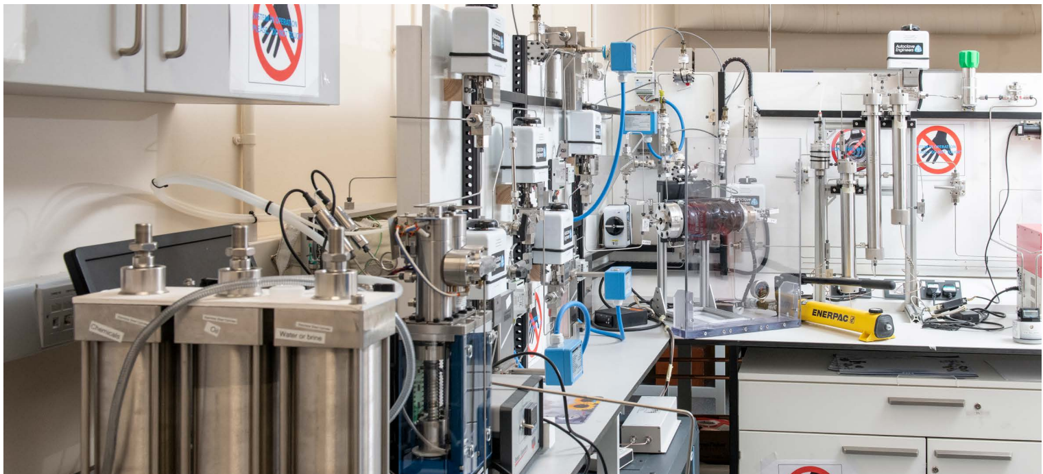
A multipurpose enhanced oil recovery (EOR) rig developed at the School of Engineering is used in laboratory studies of different recovery methods associated with chemical, thermal and gas injection processes. The rig is unique in its ability to automatically switch between different EOR techniques, separate different phases and treat downstream waste gases for storage and disposal.
