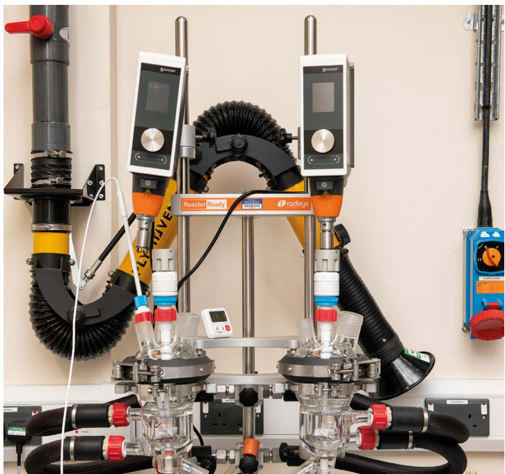
A multipurpose enhanced oil recovery (EOR) rig developed at the School of Engineering is used in laboratory studies of different recovery methods associated with chemical, thermal and gas injection processes. The rig is unique in its ability to automatically switch between different EOR techniques, separate different phases and treat downstream waste gases for storage and disposal.
