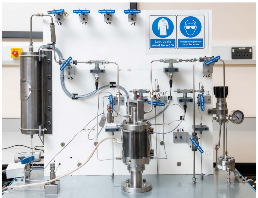
A multifunctional formation damage test rig designed and fabricated at the School of Engineering is being used to simulate practical drilling and production operation scenarios in shale, limestone and sandstone formations at reservoir conditions.
