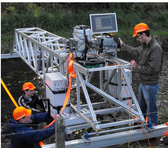
In-situ study of river turbulence in the Urie River (Scotland) using an advanced Field Particle Image Velocimetry System developed by the School.
