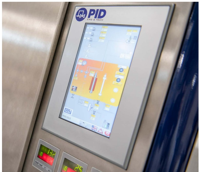
A multipurpose enhanced oil recovery (EOR) rig developed at the School of Engineering is used in laboratory studies of different recovery methods associated with chemical, thermal and gas injection processes. The rig is unique in its ability to automatically switch between different EOR techniques, separate different phases and treat downstream waste gases for storage and disposal.
