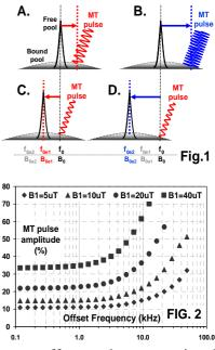
irradiation (C and D in Fig. 1). This method provides the same off-resonance effect as the conventional method, but without the complications.
