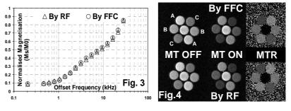
acquired by means of the FFC method (top row) and the conventional RF method (bottom row), with MT irradiation (right column) and without (left column). Due to the absence of bound protons in the control sample, the MT effect (or MT ratio) is almost zero while MT effects increase with increasing concentration of the agarose. This result also shows excellent agreement between the measurements obtained by the two different methods.
