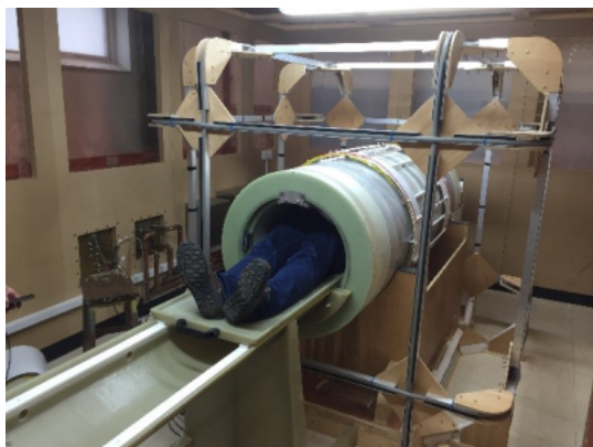
The FFC-MRI system with Earth's field cancellation coils
