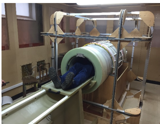
Figure 1: The FFC-MRI system and earth's field cancellation coils.
