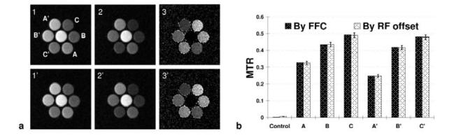
**Fig. 5.** (a) Experimental results obtained by conventional (bottom row) and new (top row) methods before (images 1 and 1') and after (images 2 and 2') MT irradiation and MTR images (3 and 3'), (b) Calculated MTR values for each component of the phantom derived from the RF offset and the FFC MTC techniques.
