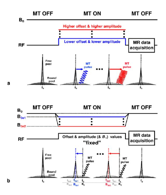
**Fig. 1.** Schematic comparison of (a) the conventional RF offset technique and (b) the novel FFC technique associated with the difference of pulse sequence timing diagrams (particularly,  $B_0$  and RF pulse lines) and the status of both spin pools with and without off-resonance MT irradiation.
