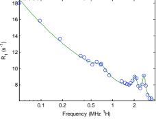
Figure 1: Dispersion curve obtained from a diseased cartilage. The quadrupolar peaks appear at 0.6, 2.0 and 3.0 MHz app.
