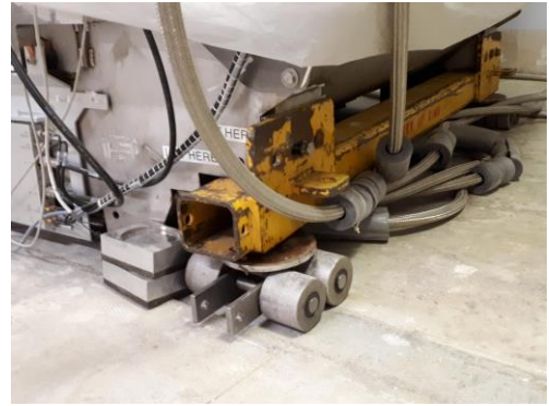
Scan room after the RF cage has been removed with a close-up of the “roller skates” used so the magnet can be moved around the room.
