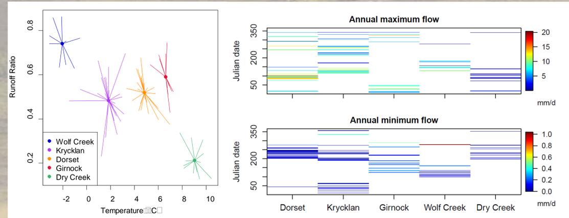
Figure 2. Comparison catchments based on observations. *Left*) Mean annual temperature versus mean annual runoff ratio. *Right*) Timing and magnitude of annual maximum and minimum flows.
