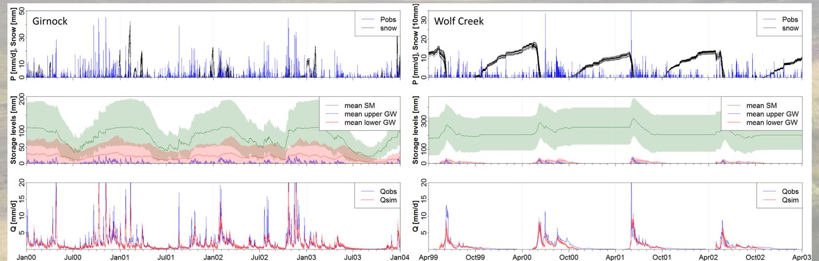
Figure 5. Examples of 4-year time series of model results for Girnock (left) and Wolf Creek (right). *Top row*) Observed precipitation and modelled snow, *middle row*) Storage levels, lines are means from 20 model runs, the coloured band indicates the range, *bottom row*) Observed and simulated discharge.
