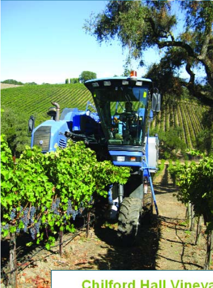
Left: Figure 1 - Mechanised Grape Picking (Harvest Pro Mechanical courtesy of Greg Kovacevich, Vineyard Ops. Inc., USA).
