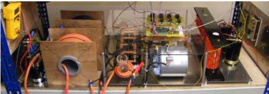
Figure 1: 30KW 200V/900V DC-DC transformer and circuit breaker prototype (2011)
