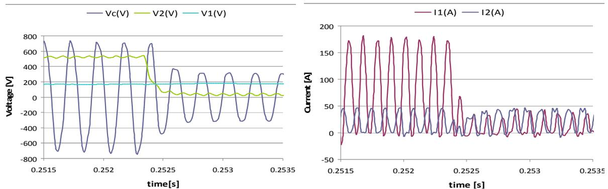
Figure 2: Prototype testing for DC faults on  $V_2=520V$  DC bus, in step up mode ( $V_1/V_2=180V/520V$ ). It is seen that the DC transformer naturally reduces power transfer and does not propagate DC faults.
