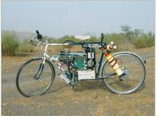
Figure 4 Fuel-cell-powered bicycle
