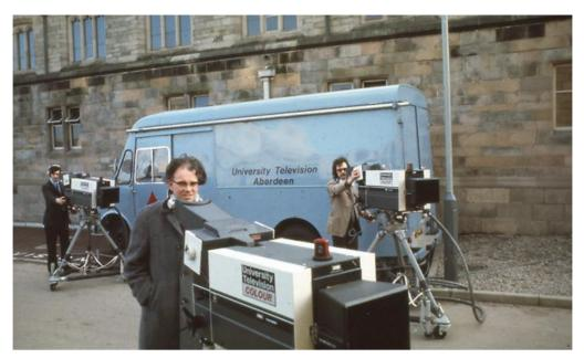
Figure 1: Scanner vehicle with its 3 EMI 2001 cameras.
