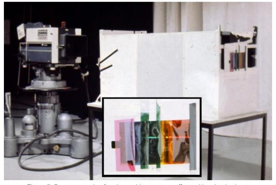
Figure 7: Box construction for observable spectrum effect, with gel strips inset
