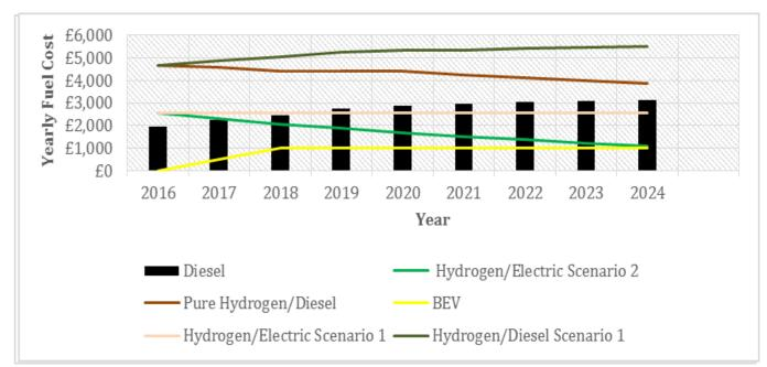
By 2018, under the assumption of continued utilisation of the *HRSs*, the yearly cost of hydrogen can equal the price of diesel. **Conclusion**
