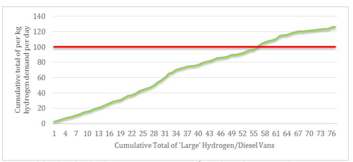
It would take the hydrogen conversion of 55 diesel powered vans, powered only by hydrogen to stimulate over a 100kg of hydrogen a day. On average these *FCEVS* contain a £30000 *TCO* premium.
