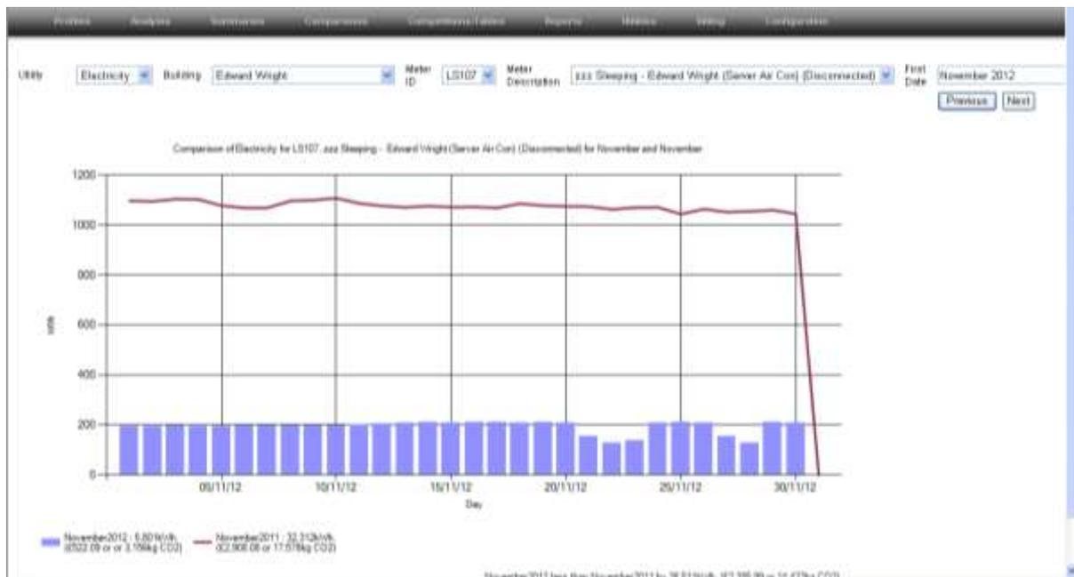
The graph above demonstrates that the electricity consumption reduced from that need for mechanical cooling to only the amount of fan power required to ventilate the data centre. Electricity use dropped from 1,100 kWh/day to 200 kWh/day or by 82%.
