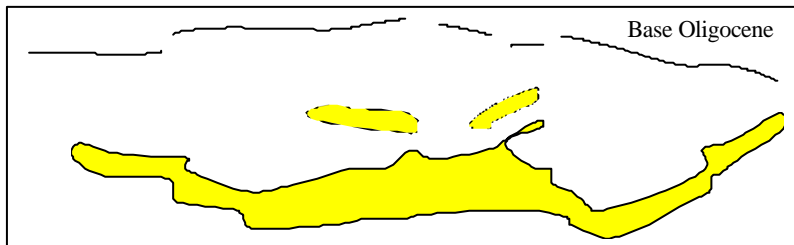
Fig. 1. Examples of injected and remobilised sand geometries imaged on 3D seismic data (data courtesy of Chevron UK and partners in the Alba Field).
