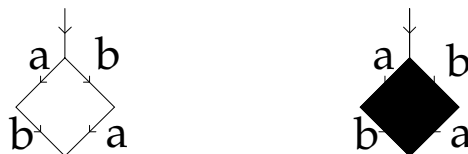
FIGURE 1. Two HDA, both modelling execution of the actions a and b . The first requires a sequential execution, whereas the second allows concurrent execution.
