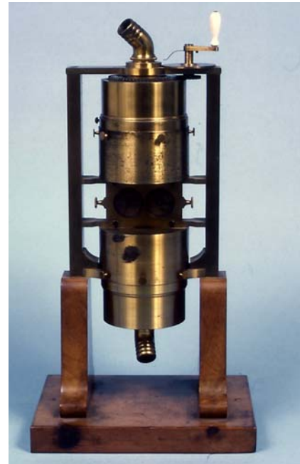
Helmholtz double siren from the 19 th century acoustic demonstration equipment of David Thomson.
