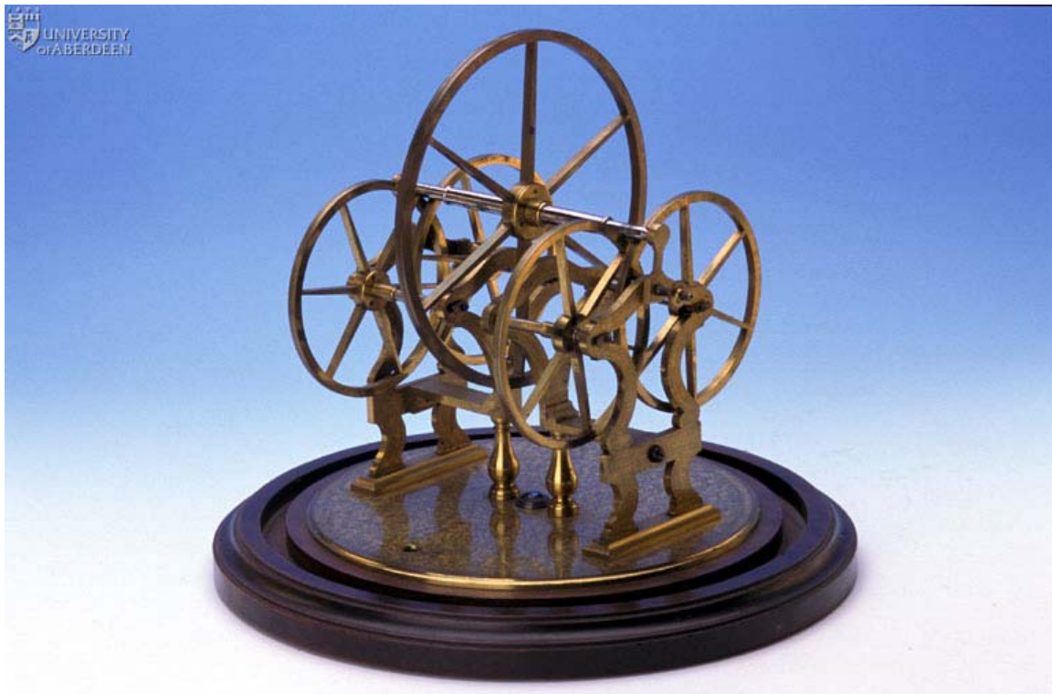
Frictionless wheels, or the next best thing prior to air bearings, from the top of an Atwood's machine made in the later 18 th century by Patrick Copland.
