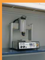
automatic dispenser for the deposition of polymeric membranes
