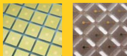
Au transducers fabricated on silicon (left) and on epoxy-glass laminate support (right)
