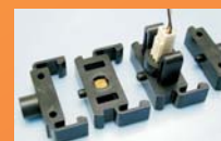
commercially available MEDBRYT's modular flow-cells for solid-state microelectrodes
