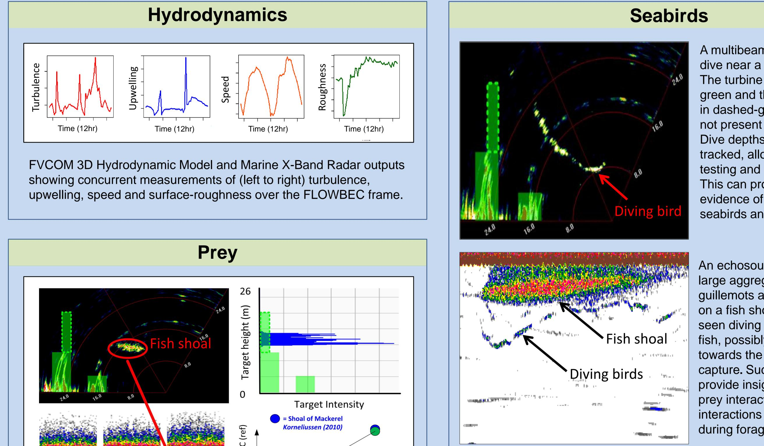
A multibeam image of a seabird dive near a tidal stream turbine. The turbine structure is shown in green and the final blade radius in dashed-green (turbine blades not present in this deployment). Dive depths and profiles can be tracked, allowing hypothesis testing and quantitative analysis. This can provide direct empirical evidence of interactions between seabirds and turbine structures.
