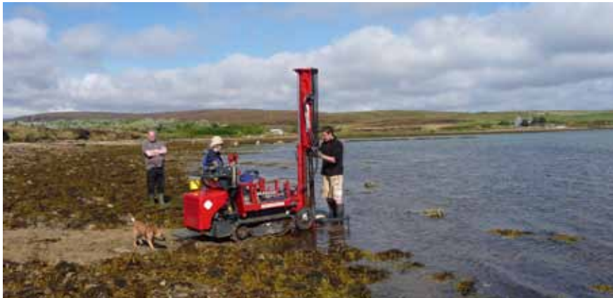
Fig. 3. Extracting cores with the terrier rig at Mill Bay
