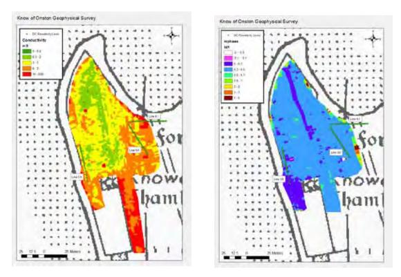
Figures 12 & 13: Ground Conductivity at Point of Onstan.
