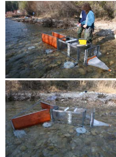
Figure 2: The portable flume: flume characteristics and dimensions, plan view of the flume with the doors in the normal position and with doors opened, increasing discharge and altering hydraulic conditions (diagram from Vericat et al. 2007). Photographs illustrate both operations.
